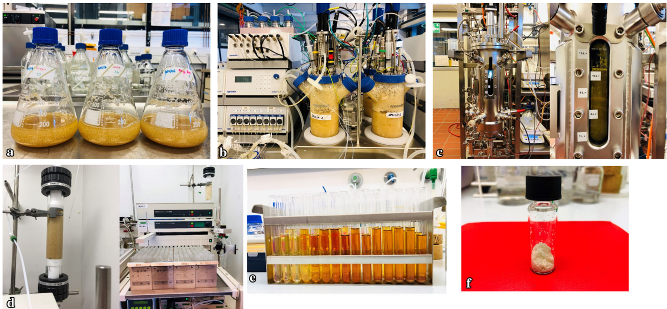
Fig. 55 Stages of the production and isolation of a biologically active metabolite from the cultures of a basidiomycete ( Omphalotus nidiformis ). a Submerged cultivation in shake flasks. b Stirred tank fermentation in a parallel 1.5 L Bioreactor systems. c Bench-Scale 10 L stirred tank. d Column chromatography for fractionation and
